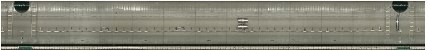
Cylindrical orthophotography of a road tunnel
