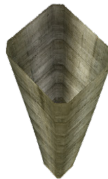
Textured 3D model of a bridge stack (internal) Square section 4m x 4m / 50m deep
