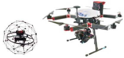
SITES drone used for inspection on photogrammetric surveys
